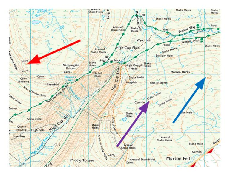
Contours show the height of the land. The closer the contours are together the steeper the land, the further apart they are the flatter the land.
