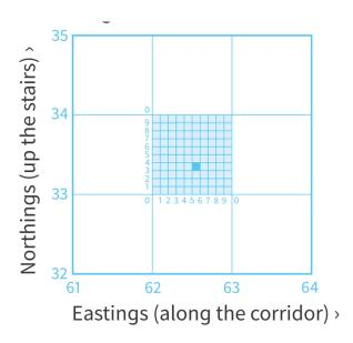
Grid references are used to identify locations on a map. There are both four figure and six figure grid references. A four figure grid reference gives a 1km square area as a location. A six figure grid reference gives a much more precise location and is much more useful when navigating and route planning.
